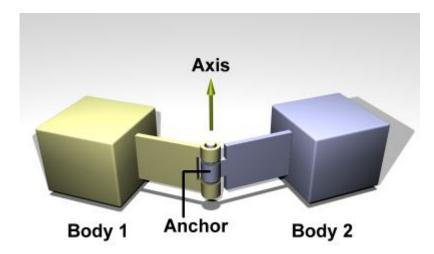
This joint is used to model things like doors and wheels (picture turning the axis 90 degrees to the left, the bodies will now spin around each other).
