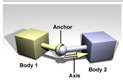
This joint is used to model things like rope segments and arm joints
