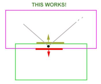
As seen in the image above the player is inside the bounding box of the purple room as well so it doesn't have to have to see the portal. The dark yellow rectangle is where the portal in the purple would be placed.
