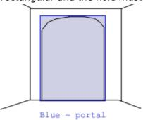
The portal must be placed in the "\_room#" group that it belongs to. The normal of the rectangle must be facing the center of the room it belongs to and **not** the room it connects to.
