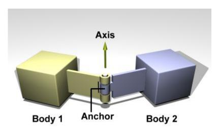
• Min Angle & Max Angle: Maximum and minimum angle between the bodies relative to the start position. Max angle is in the positive direction and min in the negative. To get the positive direction place your thumb on your right hand in the direction of the axis. Now bend your fingers towards your palm, the direction in which you fingers are pointing is the direction of the positive angle. In mathematics this is called the right hand rule. Valid values are 0 - 179.
