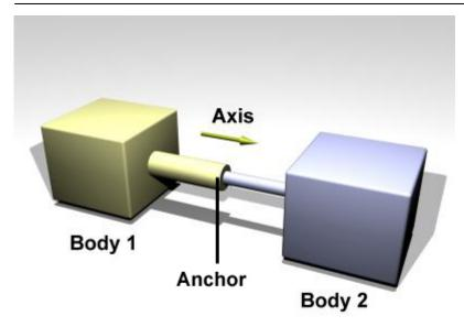
• **Min Distance** & **Max Distance**: Picture the anchor as attached to Body1(Parent). When the anchor is moved in the distance of the axis the distance gets larger and when it moves in the other way it gets negative (and smaller). At the start position the distance is 0.
