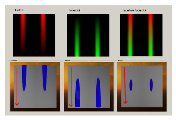
When saving the texture it should be exported as a compressed 3dc dds. If the quality for the texture is not good enough then the texture can be saved as a tga, for this to work the red channel has to be copied in to the alpha channel and the green channel to the blue channel.
